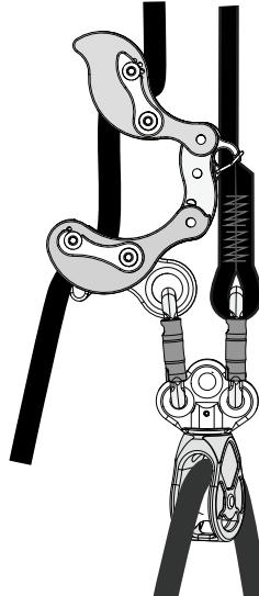
Rock Exotica recommends separating the Akimbo and termination end of the rope. The Rock Exotica Hydra is one example of a suitable connection. Connect the Akimbo using an appropriate oval carabiner. Rock Exotica recommends a RockO WireEye carabiner
