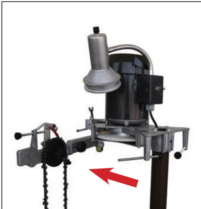
Swing the arm around to the other side when all the cutter-teeth on one side are sharp. This will allow you to sharpen the cutter-teeth on the other side.
