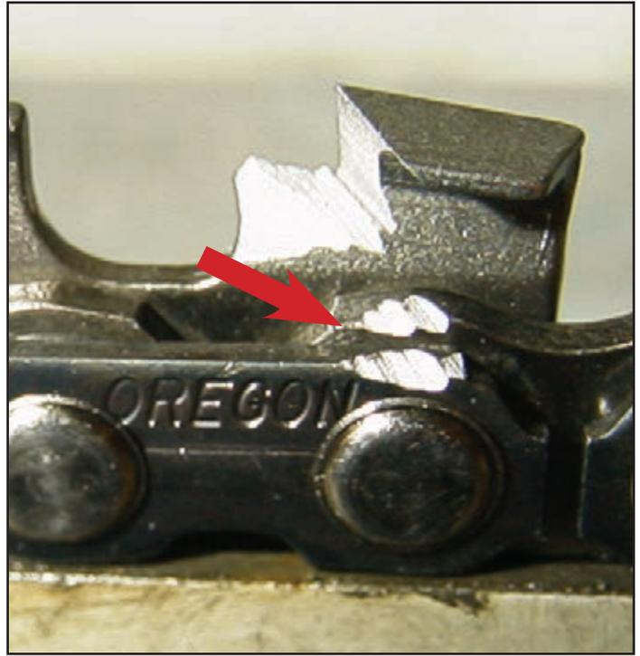
If the edge-thickness of the grinding wheel is too great and/or the grinder is not set up correctly, the chassis of the cutter-teeth can be damaged during sharpening.
