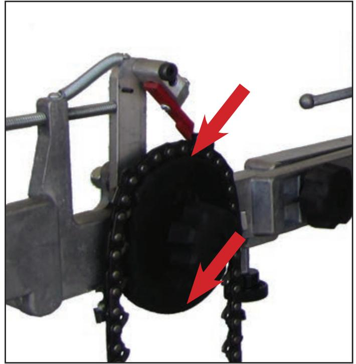
This grooves in this disk are .050" on one side and .063" on the other. Position the groove that matches your chain up. It can tilt slightly forward like this one if you wish. The exact position does not affect the grind angles.
