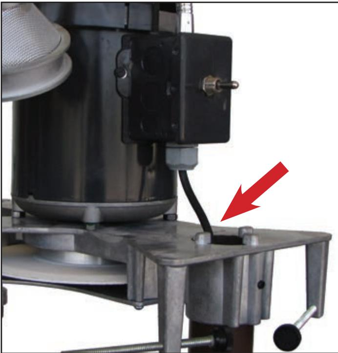
Feed the power-cord down the top of the stand-post. This keeps the power-cord out-of-the-way of the grinding operation.
