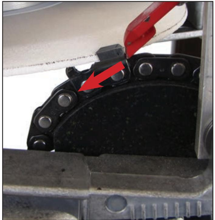
As cutter-teeth become shorter, it is necessary to advance to red stop-pawl to achieve corner alignment. As a consequence, the cutter sits further down the arc, and the inside-top-plate angle becomes more blunt. To compensate for this, the arm holding the chain-guide can be set lower when sharpening chains with short cutter-teeth.
