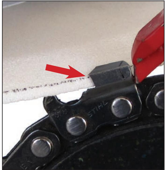
Before you turn the motor on, make sure nothing is touching the grinding wheel. Notice the corner of the wheel is aligned with the outside corner in the cutter-tooth. This is what you need to accomplish.
