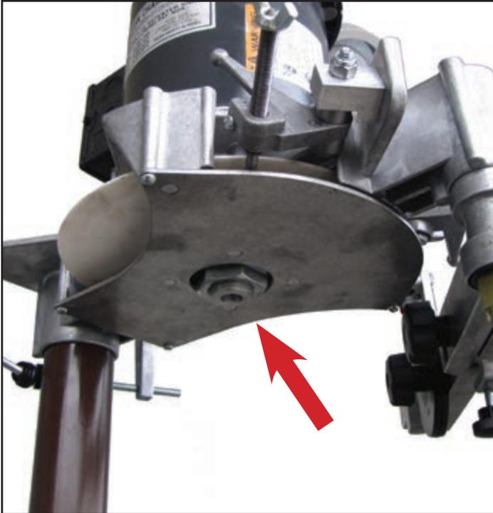
When replacing the grinding wheel, be sure to replace the wheel guard.
