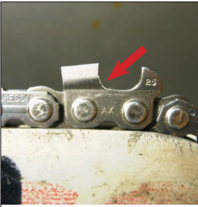
The gullet on this cutter-tooth has been ground out. Gullets can be removed with a round grinder or round file. The Simington #451C does not remove gullets, but they need to be removed for a sharp square-chisel chain to perform well.
