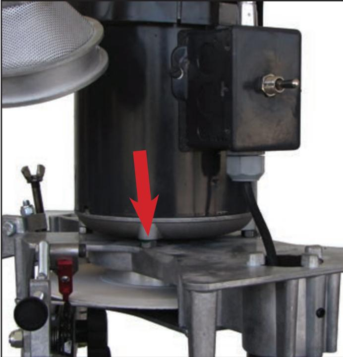
This is one of four motor-mount posts that can be shimmed to match the plane of the wheel to the sweep of the swing-arm. These planes need to match or the grinder will not produce similar angles on right-hand and left-hand cutter-teeth.
